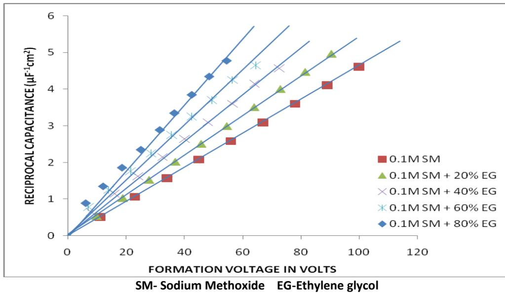
Table- 1: Effect of solvent on the Anodization of Zr-Nb in 0.1 M Sodium Methoxide (SM)
