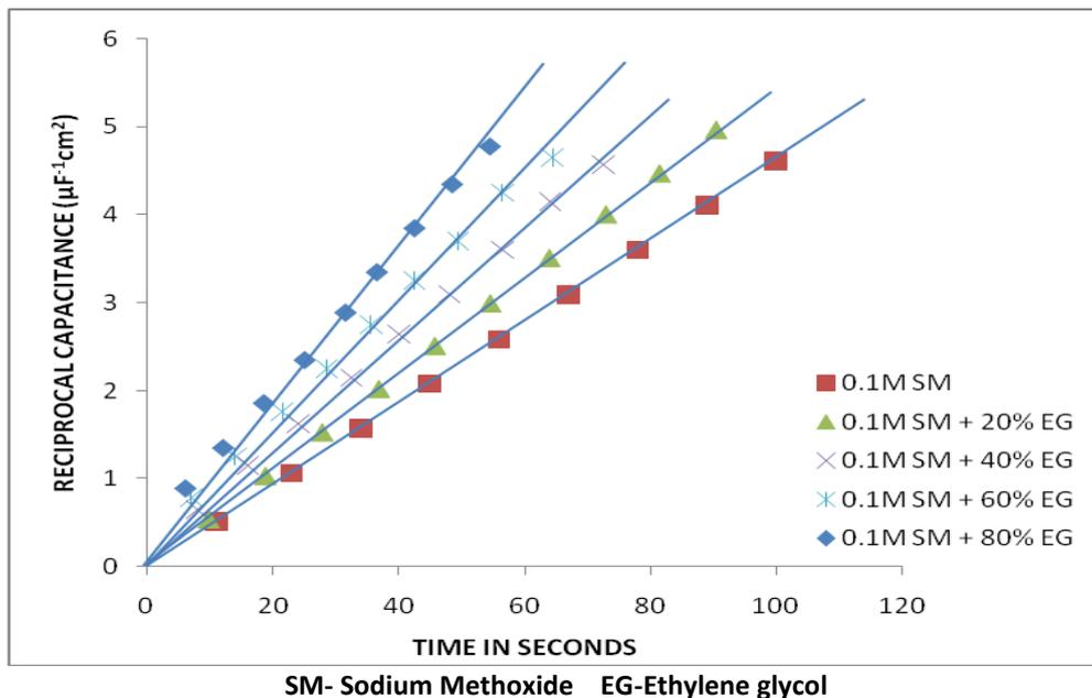
Figure 3: Plot of Reciprocal Capacitance as a function of Formation voltage in aquo-glycolic Solution
