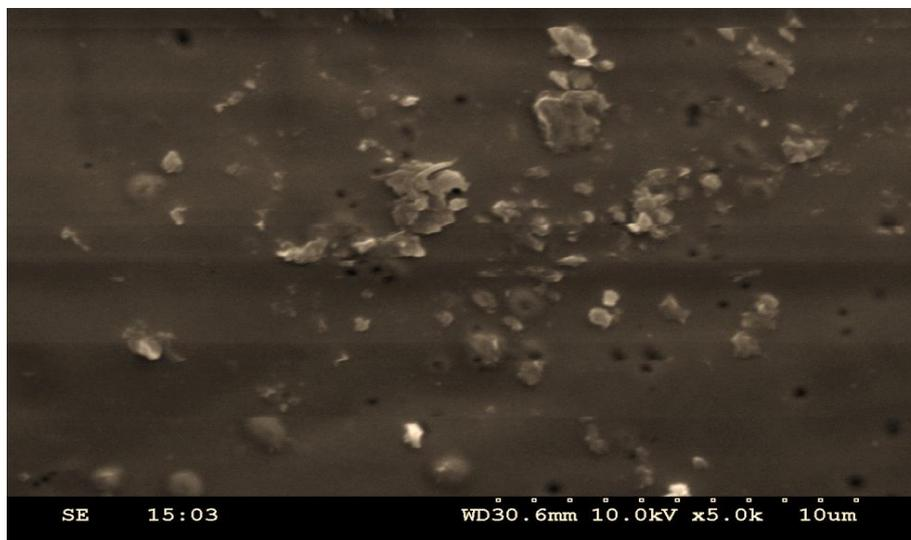
**Figure 5: SEM of the film formed upto 220V in 0.1M Sodium methoxide (Aquo-glycolic medium) at room temperature (Magnification of the micrograph is X 5000)**
